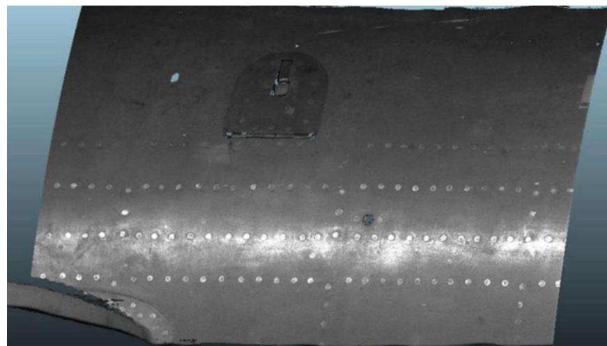
Measured point cloud of an aircraft skin
