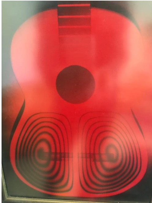
Time-average hologram of a vibrating guitar. Around 1970.
