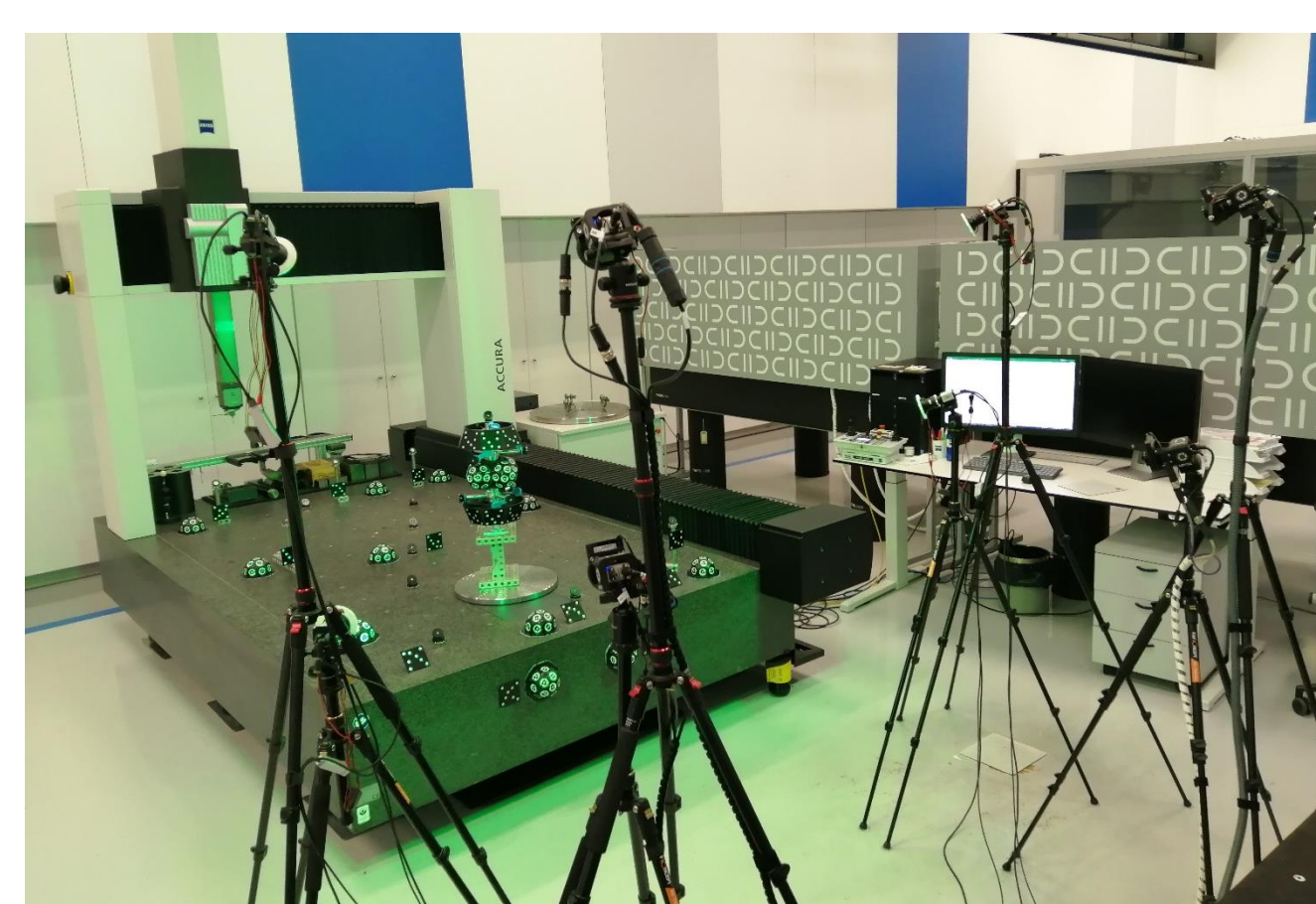
Fig 8. CMM testing at IDEKO
