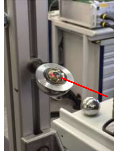
1.5" SCE -Reflector tilt upwards
