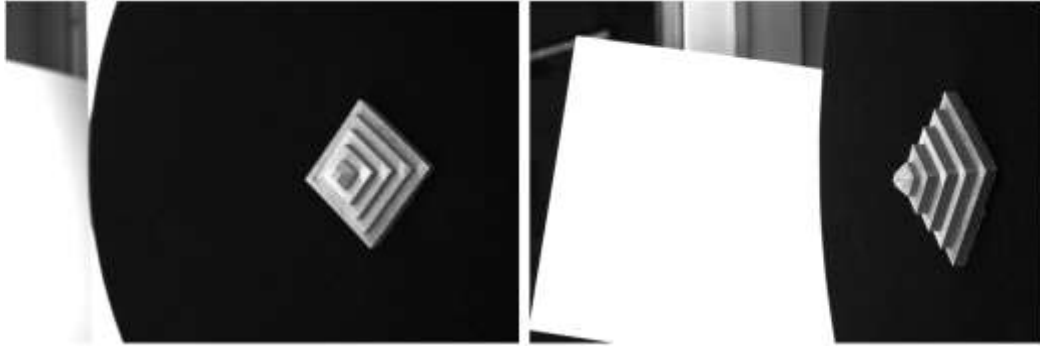
Stereo images: a pyramid artefact is captured from each camera
