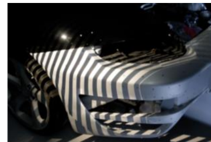
Analysis of gray code measurements for each pixel
