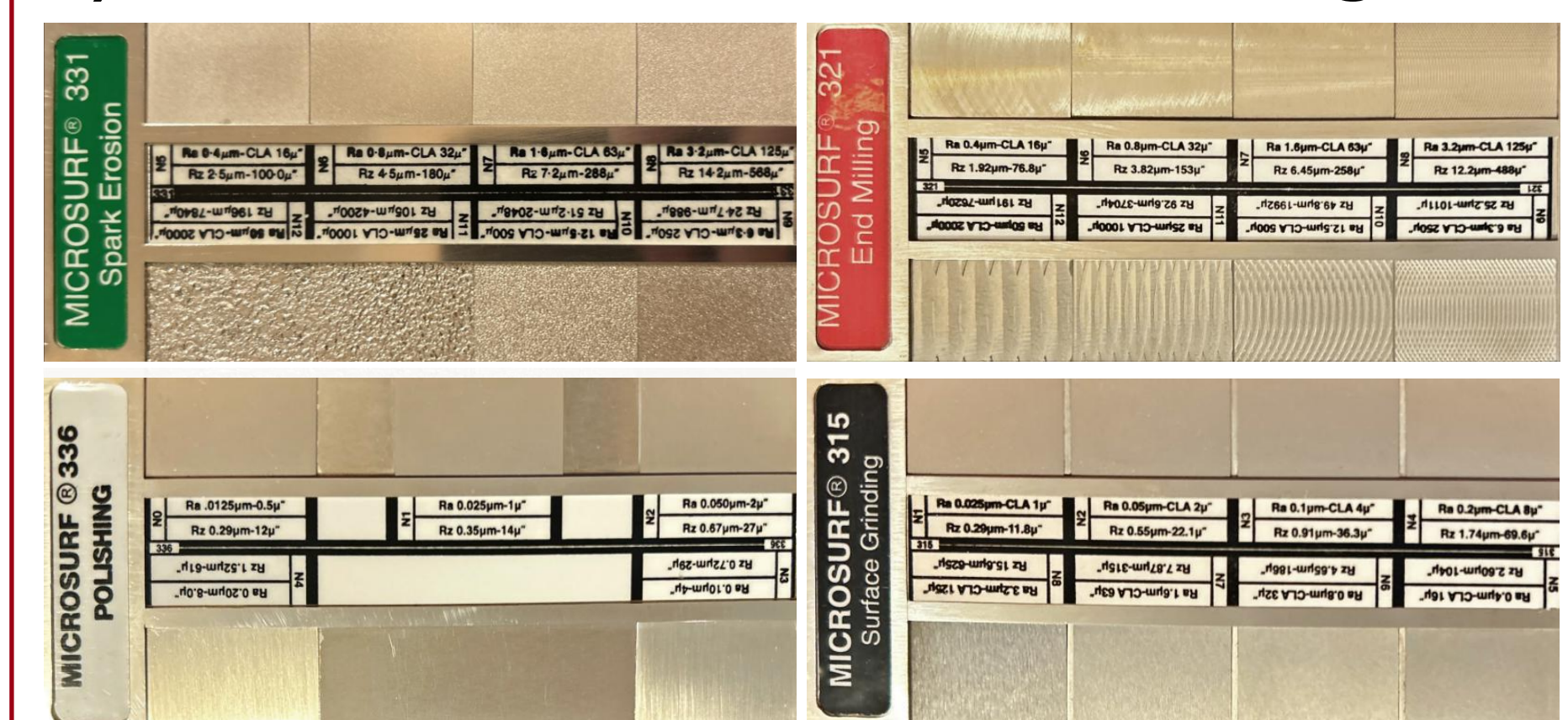
Fig. 5. Roughness test specimens with different machining and range of surface roughness levels
