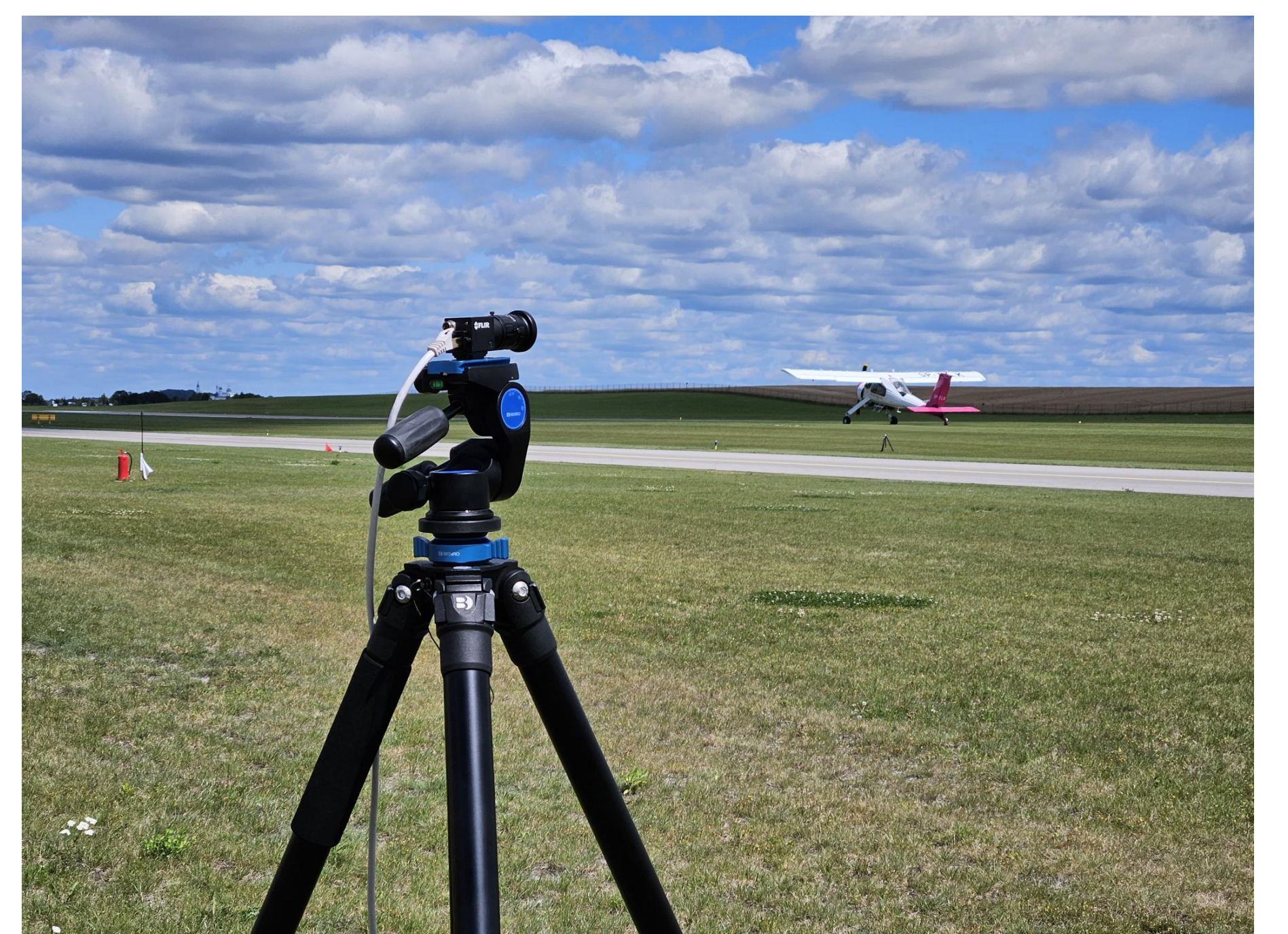
Figure 5. Measurement campaign to determine aircraft landing positions for the validation of the IMUMETER system.
